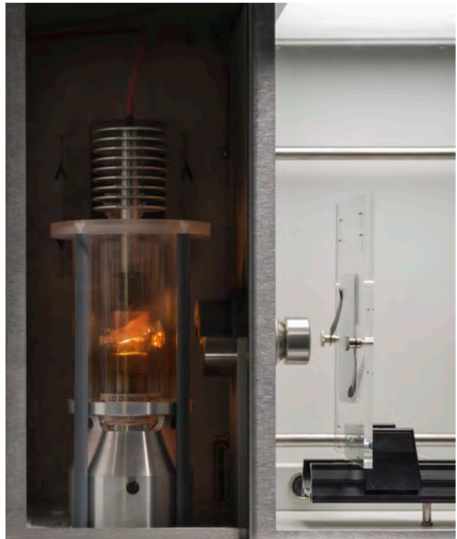
Creation of a Laue diagram on X-ray film.
