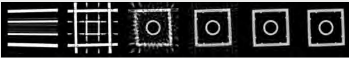
The CT algorithm seen in action: The images show the same sectional image of a LEGO brick after the back projection from 1, 4, 15, 45, 90 and 360 angles.
