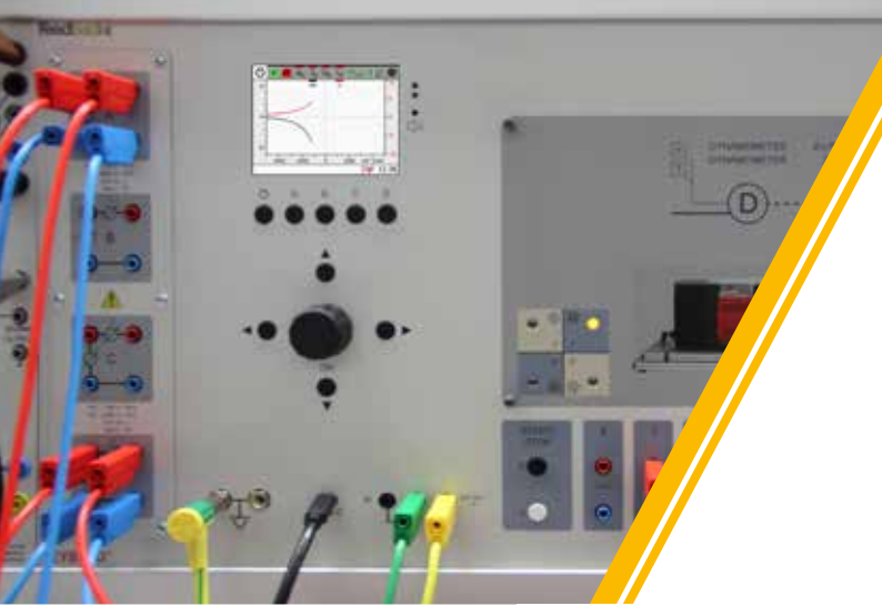
Characteristic curve of a series motor (left-hand rotation)
